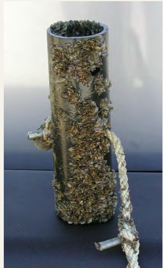
FIGURE 1. ABS pipe covered with quagga mussels. Photo courtesy of California Department of Fish and Game.
